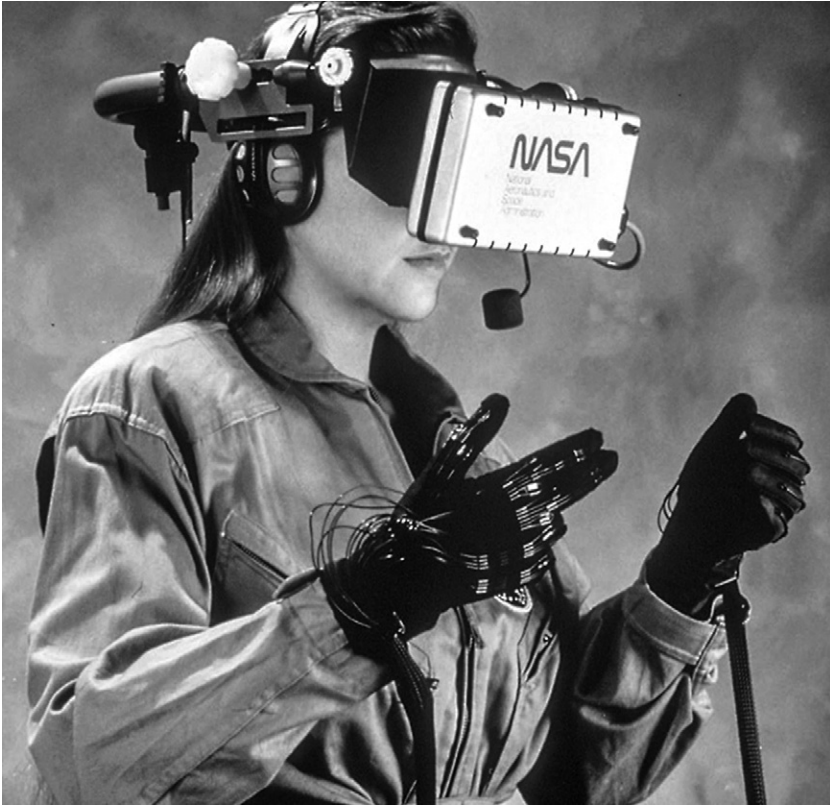
Figure 6.2 NASA Scientist Sally Rosenthal demonstrating the VIEW VR System in 1989, including the DataGlove interface developed by VPL. Source: Photograph by Wade Sisler.
