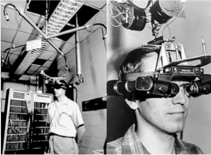
Figure 5.1 Ivan Sutherland's Sword of Damocles head-mounted display, widely considered the first VR headset. This system utilized mechanical pivots to provide the viewer with six degrees of freedom in the head mount for an immersive viewing experience.
