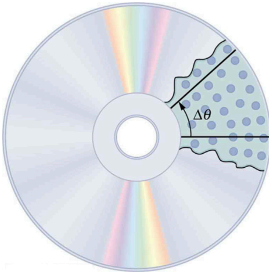
Figure 13: All points on a CD travel in circular arcs. The pits along a line from the center to the edge all move through the same angle \Delta\theta in a time \Delta t
