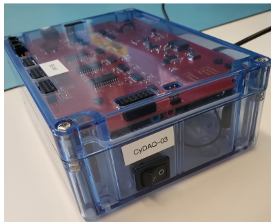
(a) The CyDAQ with power switch visible on the right side.
