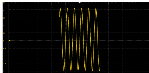
Figure 3.11: Scope for Time Base 200 \mu\text{s}/\text{div} . The signal appears cut off.
