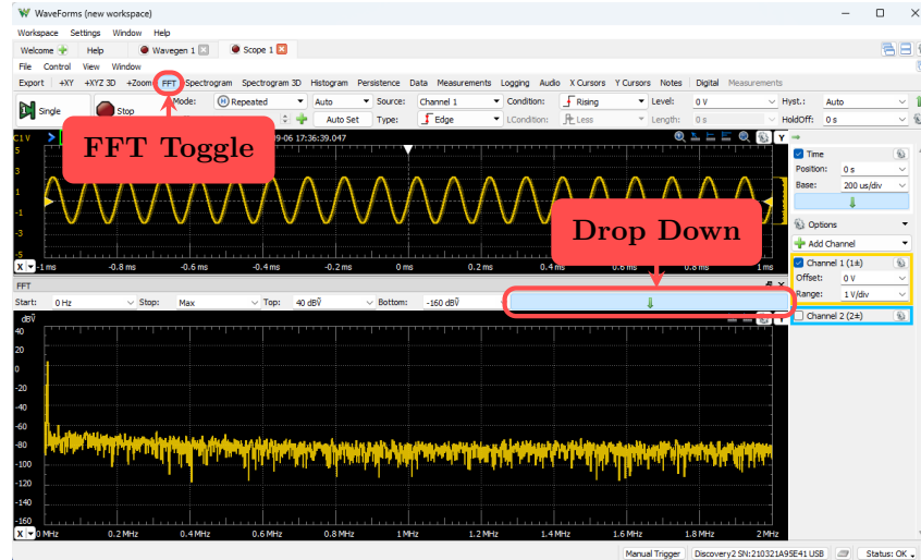
Figure 3.12: Scope with FFT View visible. The FFT Toggle and Drop Down for the FFT View are highlighted.
