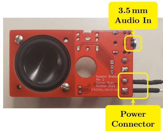
Figure 10.8: CyDAQ Speaker showing 3.5 mm Audio terminal and Power Connector .
