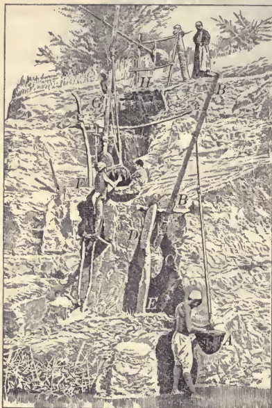
FIG. 23. AN EGYPTIAN SHADOOF , THE OLDEST OF WELL SWEEPS, IRRIGATING THE FIELDS
