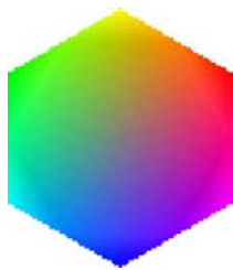
Fig. 15.3 The color hexagon used for analyzing the color content of the PCA and ICA features. The hexagon is the projection of the RGB cube onto a plane orthogonal to the luminance ( R + G + B ) vector. Thus, achromatic RGB triplets map to the center of the hexagon while highly saturated ones are projected close to the edges
