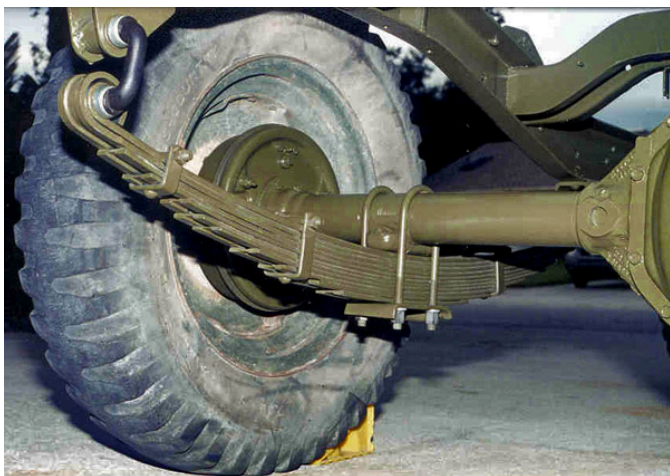
Leaf springs are often used in automotive applications to support the wheel axles.
