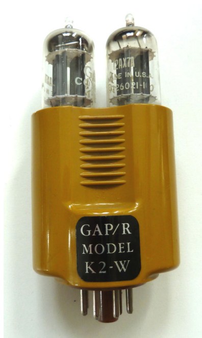
Figure 8.1: K2-W commercial vacuum tube operational amplifier (1952).
