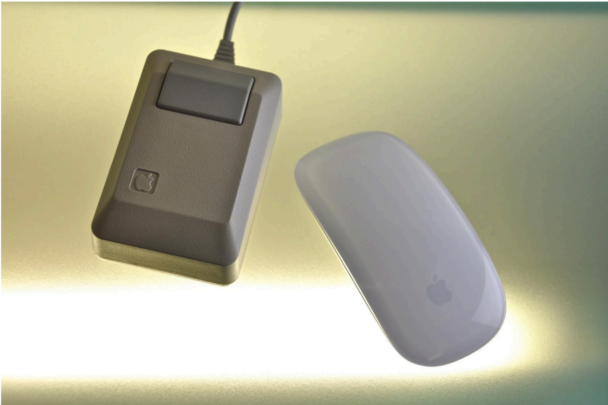
Figure 1.17 An Apple Macintosh Mouse M0100 Beige from 1984 (left), and an Apple Magic Mouse from 2009 (right) (credit: Photograph by reneko via flickr / CC BY 2.0)
