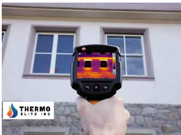
Figure 4.4: Thermographic inspection illustration.
