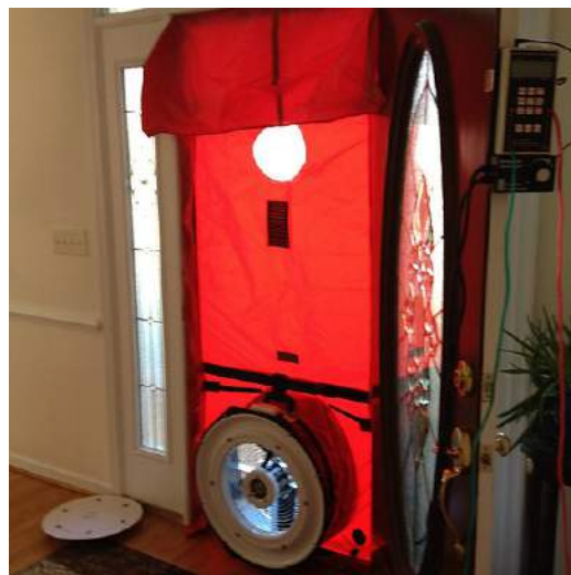
Figure 4.3: Blower door test illustration. Image description.
