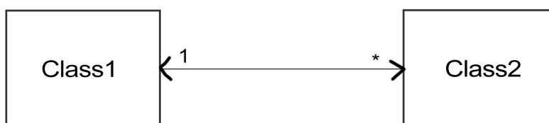
Figure 4.9 Bidirectional Association and Target/Source Multiplicity
