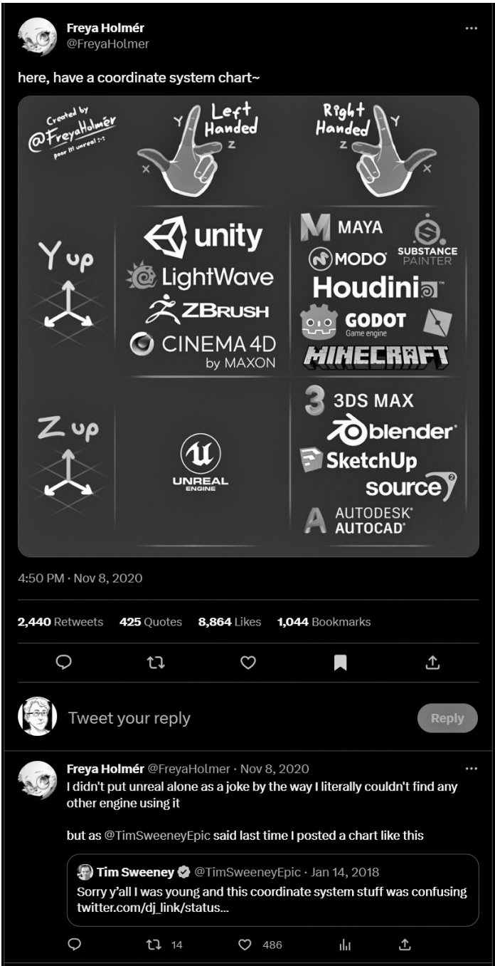
2.4 Freya Holmér’s (@FreyaHolmer) breakdown of the crossing of Y-up/Z-up and handedness orientations in popular modeling, animation, development, and play software. Unreal Engine is the only software to reflect a left-handed, Z-up coordinate system ( https://twitter.com/FreyaHolmer/status/1325557466529210369 ). Reprinted with the permission of Freya Holmér. Copyright © Freya Holmér 2020.
